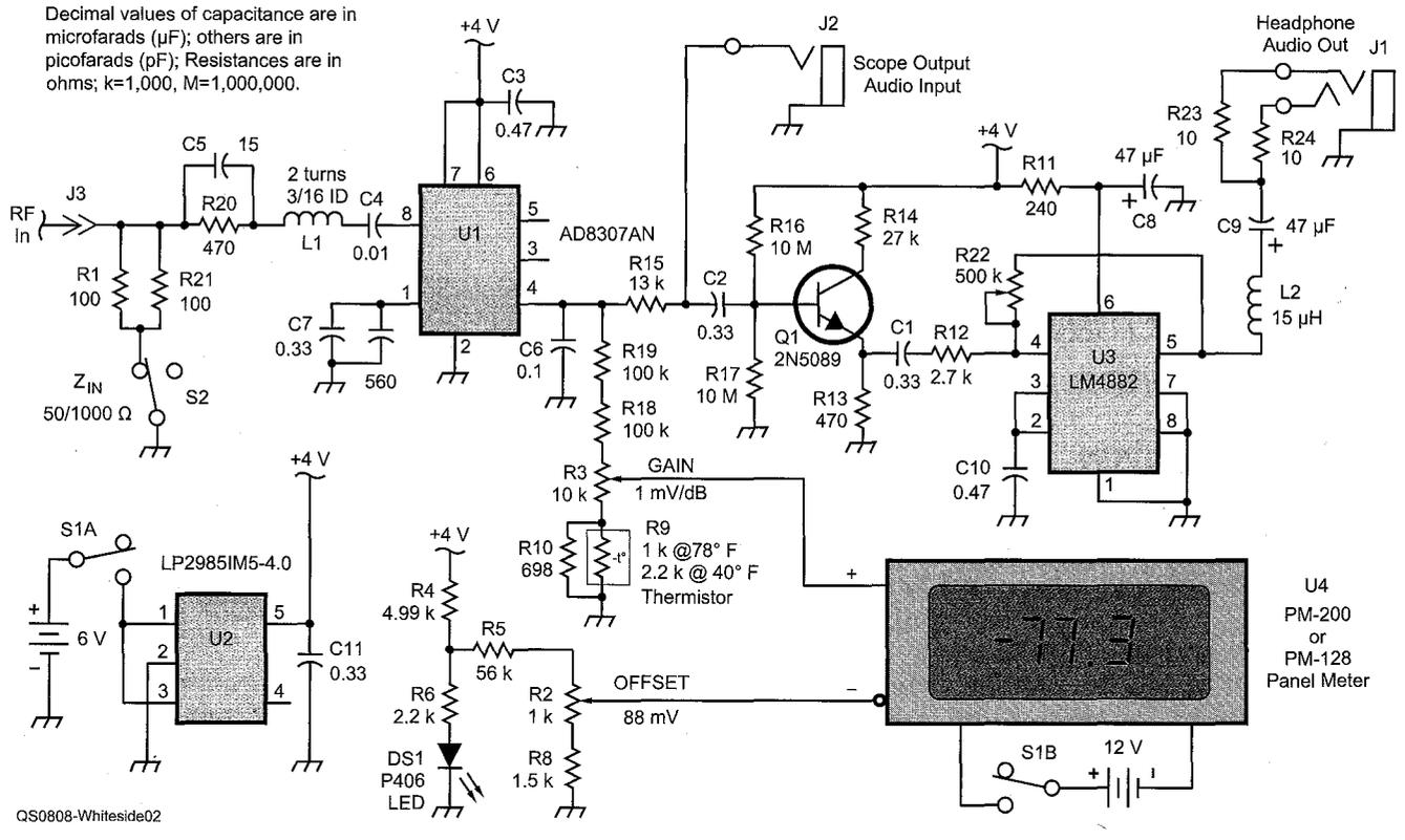
**Figure 2** — Schematic of the pocket dBm RF power meter. All resistors are 1/4, 1% metal film, most from RadioShack assortment 271-309. The audio amplifier section uses 5% resistors. All Electronics is found at [www.allelectronics.com](http://www.allelectronics.com), Chaney Electronics at [www.chaneyelectronics.com](http://www.chaneyelectronics.com) and Digi-Key at [www.digkey.com](http://www.digkey.com).
