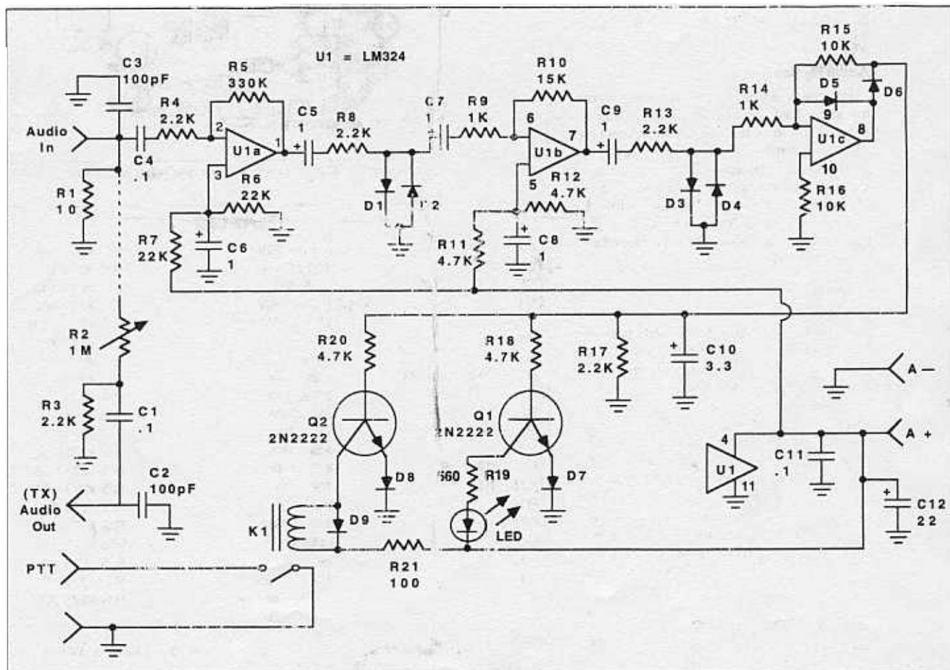
Figure 1. Schematic for PTT control from receiver audio
