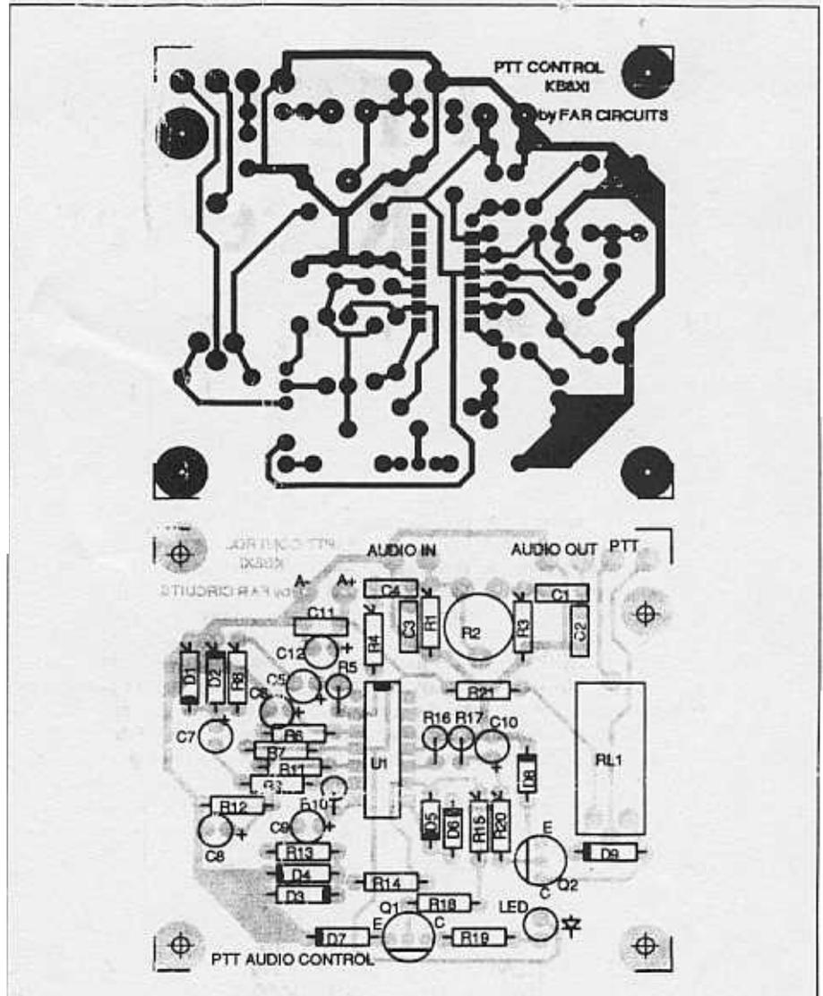
Figure 2. PC board etch pattern and parts placement.
