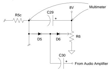
Measure  $V_{C29}$  (dc) with the function generator set at 0.1 V<sub>rms</sub> and then at 3 V<sub>rms</sub> as used in Prob. 33.A. This difference in voltage can be used to predict the recovery time  $\Delta t$  as
