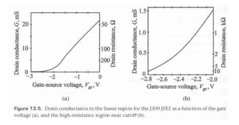
4. When the control voltage (anode of D5) decreases, then  $V_{gs,Q2}$  becomes more negative. From Fig. 13.5 we see that  $r_{ds}$  increases, which implies more attenuation of the audio signal passing through Q2 (and Q3) from U2 (Product Detector) to U3 (Audio Amplifier). Neat!
