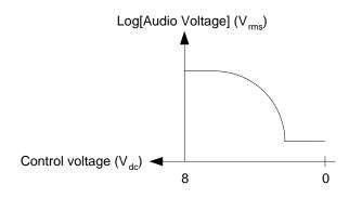
You'll plot the RMS audio voltage (speaker voltage) versus the dc control voltage (anode of D5). How do you vary this control voltage? Simply adjust R6, the AGC threshold.
