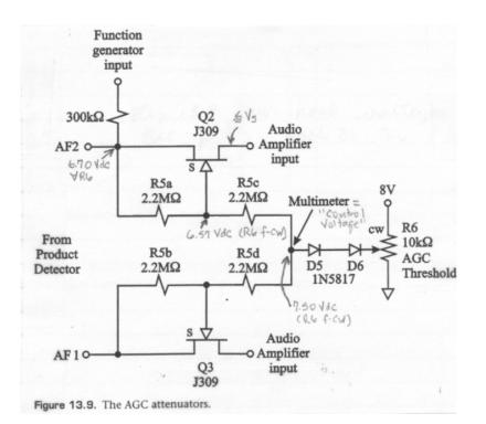
Also shown in this figure are the dc node voltages I measured in my radio with R6 fully CW.
