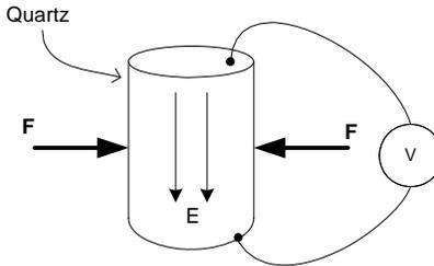
Electric starters for gas furnaces, water heaters and grills use such a piezoelectric effect.
