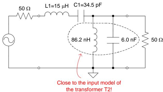
While this example was seemingly just an exercise, believe it or not, the actual RF Filter in the NorCal 40A is a two-element Butterworth bandpass filter!  $L_1$  and  $C_1$  are the series  $L$  and  $C$ , but where is the parallel  $L$  and  $C$ ?
