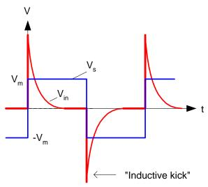
This rapidly changing current in an inductor can produce enormous  $V_{\text{in}}$  (=  $V_L$ ). Sometimes this is useful, as in an automobile spark ignition (see Fig. 2.19).
