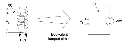
Recall that as  $V_s$  goes from  $V_m$  to  $-V_m$ , there will be a rapid decrease in I(t). It's not an instantaneous change from  $V_m/(R_s+R_L)$  to  $-V_m/(R_s+R_L)$  because of L, but a rapid change.
