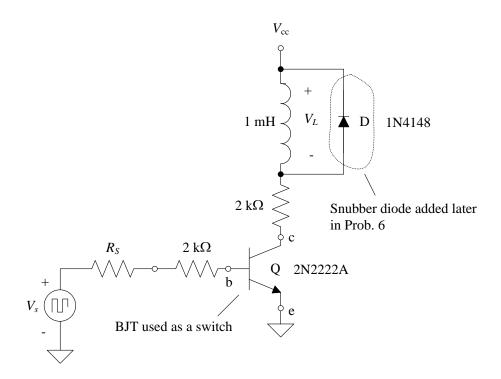
When Q turns off, there would be a very large and negative voltage  $V_L$  if D were not present. This large voltage appears across c and e of Q. If this voltage is too large, then Q could be damaged. (Think of L as an equivalent inductance of an electric motor, for example.)
