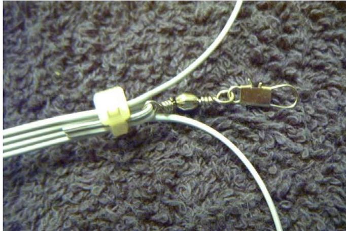
4. Secure the whole thing by wrapping the tie wrap around the feedline and loop. (Dennis Foster showed me this idea)
