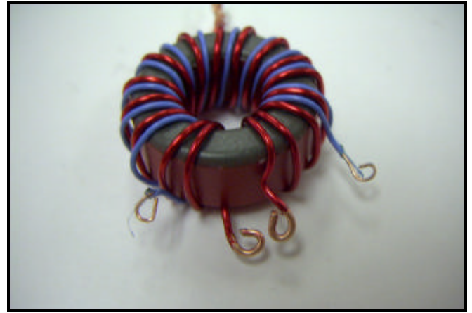
Fig. 27 – L2 and L1 both wound on the red toroid.
