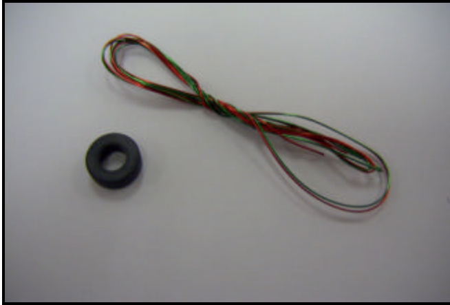
Fig. 3 – Small Toroid + Wire
