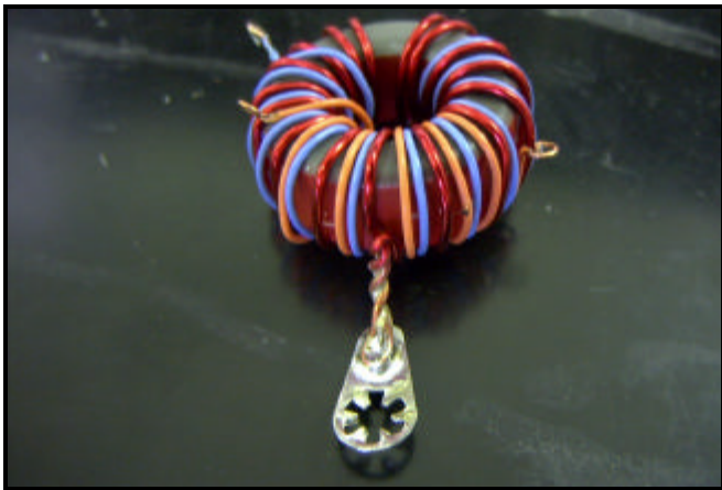
Fig. 29 – The large toroid prepared for mounting.
