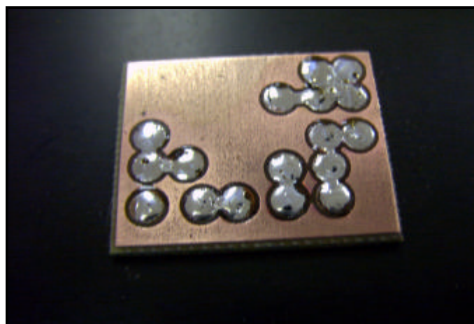
Fig. 2 – The Tinned Board
