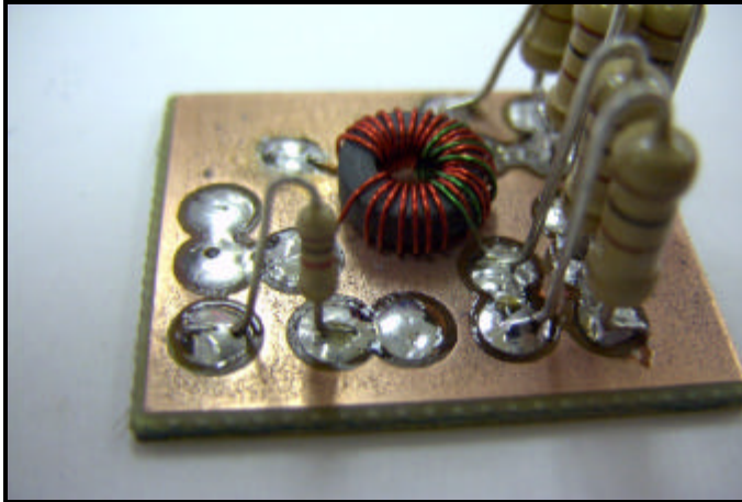
Fig. 12 – R4 soldered in place just to the left of the toroid.
