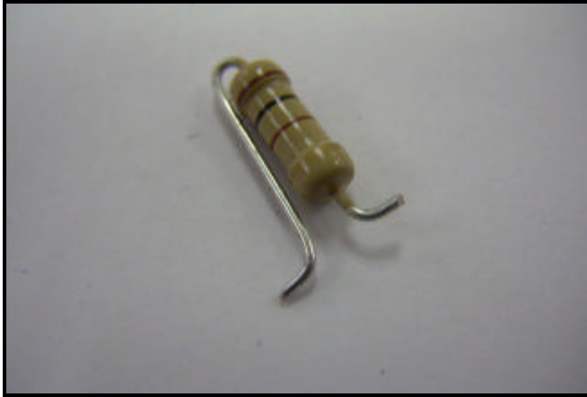
Fig. 7 – 100 ohm Resistor ready to mount
