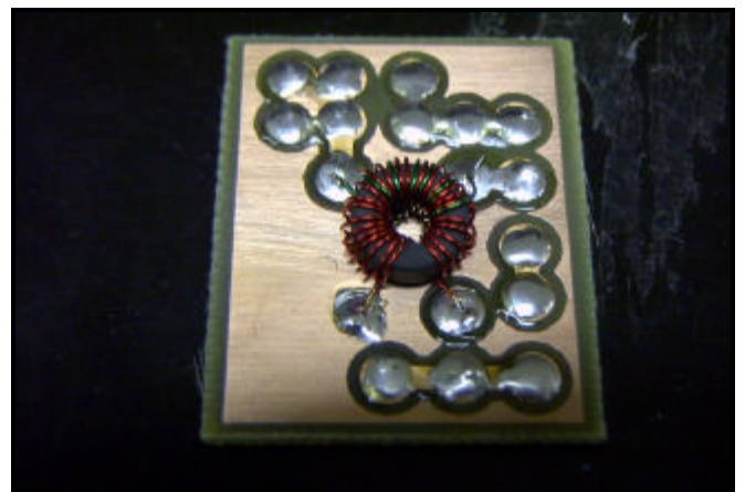
Fig. 6 – Toroid Mounted on Board
