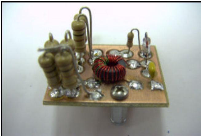
Fig. 18 – The board mounted on standoff.
