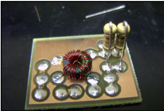
Fig. 8 – Resistors R2 & R2A Mounted.
