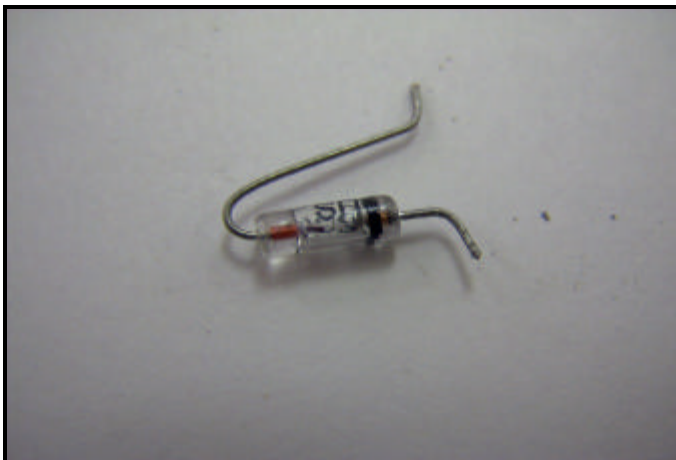
Fig. 13 – Diode D1 prepared for soldering.
