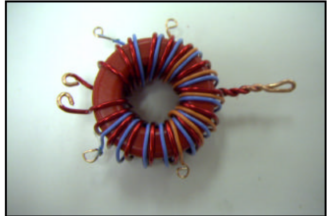
Fig. 28 – The finished Toroid, note the tap on the right side.
