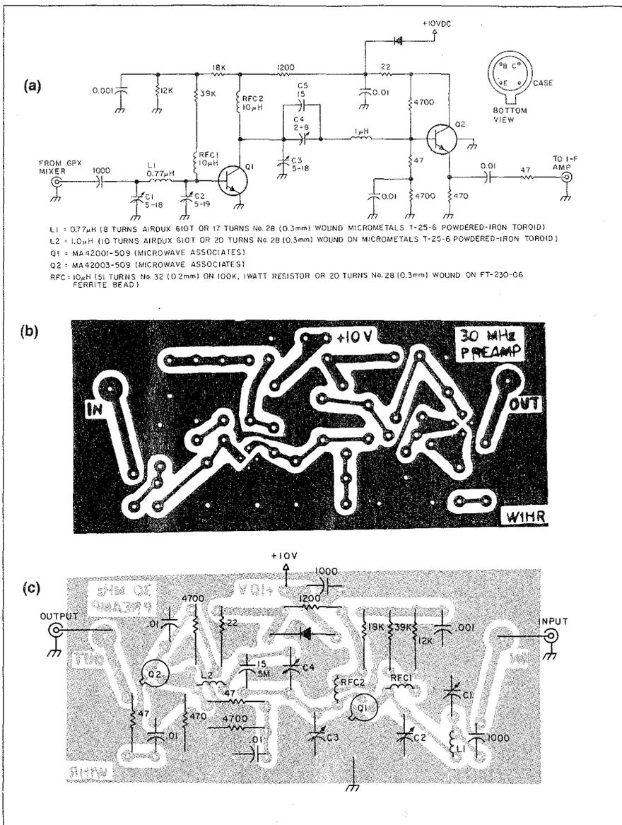
Fig. 5. 30-MHz i-f preamplifier (a) schematic, (b) circuit board, foil side, and (c) parts placement. Courtesy of Ham Radio Magazine, J. R. Fisk WIHR, October, 1978, p. 38.
