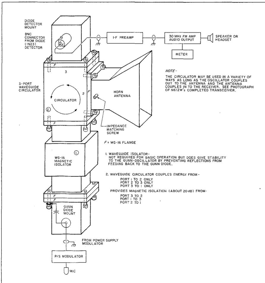
Fig. 1. Waveguide circulator 10-GHz transceiver.
