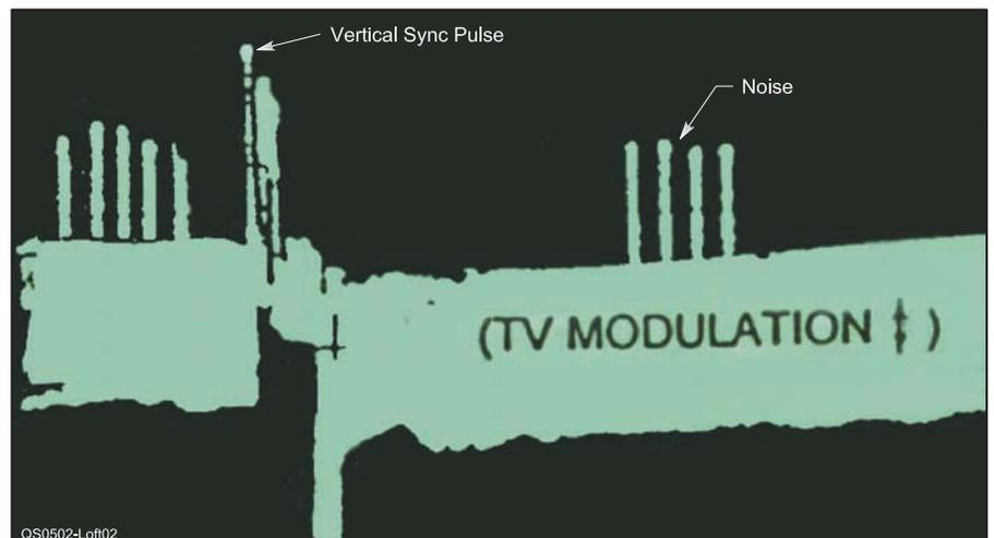
**Figure 2—An NTSC channel 5 television video pattern, at the vertical rate (59.94 Hz). The noise pattern can be clearly seen.**
