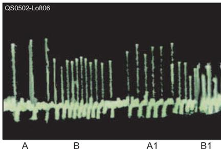
**Figure 6—Two noise patterns, representative of two power line noise sources. Patterns A and A1 are both half-cycles of one pattern; B and B1 are of another pattern.**
