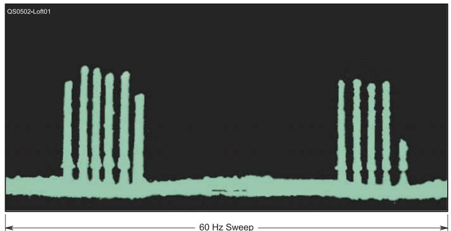
**Figure 1—Power line noise pulses detected at 75 MHz, about 2 MHz below the NTSC channel 5 television video carrier.**
