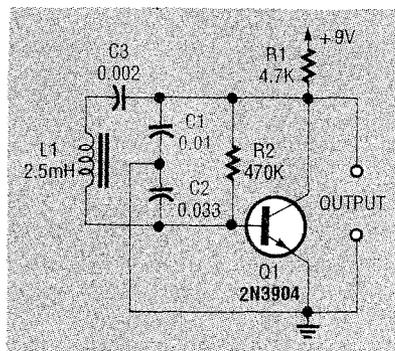
FIG. 9—CLAPP OR GOURIET LC oscillator produces an 80-kHz output.
