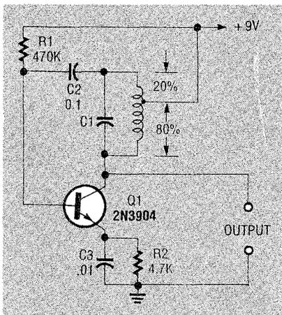
FIG. 7—SIMPLE HARTLEY LC oscillator.
