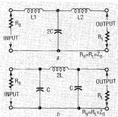
FIG. 14—LOW-PASS LC FILTERS: T-section schematic, a, and  $\pi$ -section, b.
