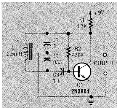
FIG. 8—COLPITTS LC OSCILLATOR produces a 37-kHz output.
