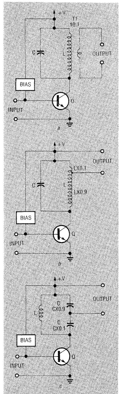
FIG. 5—LC TUNED AMPLIFIERS with low-impedance outputs: transformer coupling, a, auto-transformer coupling, b, and capacitive-divider coupling, c.
