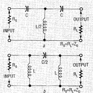
FIG. 15—HIGH-PASS LC FILTERS: T-section schematic, a, and  $\pi$ -section, b.
