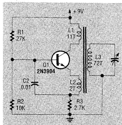
FIG. 10—SIMPLE REINARTZ LC oscillator.
