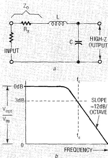
FIG. 12—TRUE L-TYPE LOW-PASS filter: schematic a, and frequency response curve, b.
