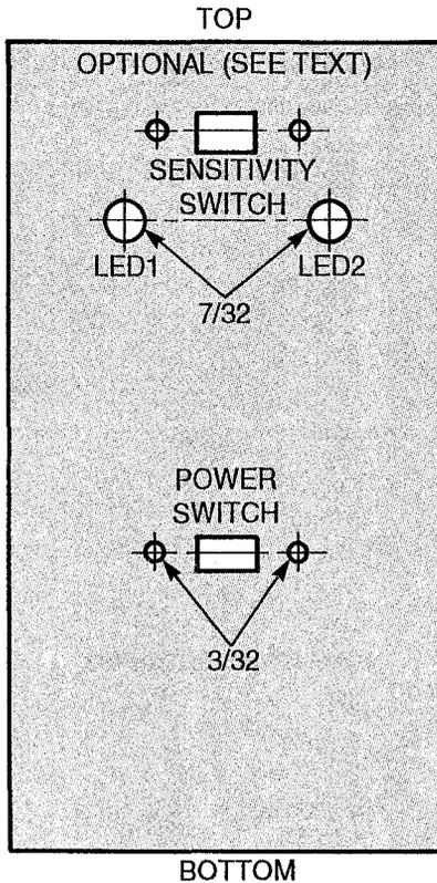
FIG. 3—DRILL GUIDE. S2 is optional, so don't drill holes for mounting it if you're not using it.
