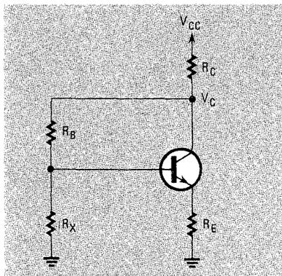
FIG. 5—THIS CIRCUIT is one of the many variations of the two basic bias circuits.
