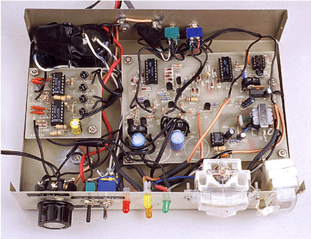
Figure 5—An inside view of one DF unit built into a 2×8×5-3/4-inch (HWD) box. Because of the height restriction, the two 4700- $\mu$ F damping capacitors (C8 and C10) are not mounted on the PC board, but near the rear panel behind the smaller of the two PC boards. One of the 4700- $\mu$ F damping capacitors is a standard electrolytic, the other is a parallel combination of five 1000- $\mu$ F, 6.3-V bipolar (nonpolarized) capacitors wrapped in electrical tape (see Note 3).
