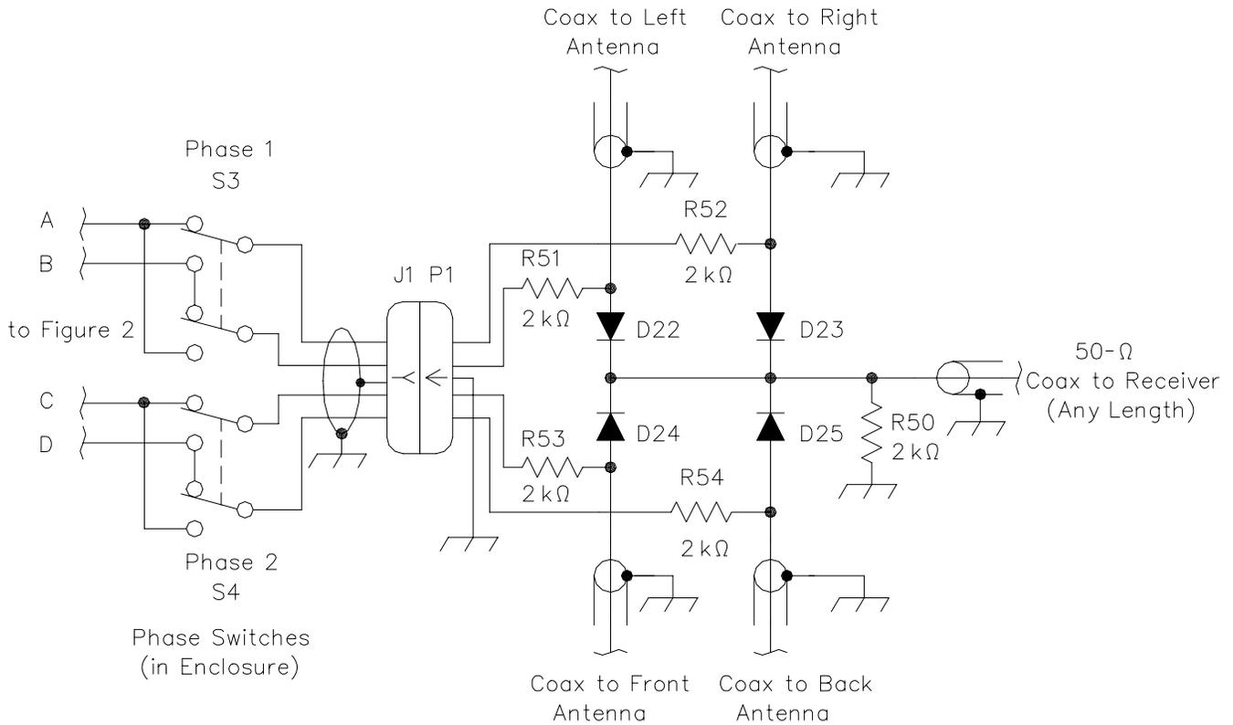
Figure 3—Schematic of the antenna switch board. Part numbers in parentheses are Radio Shack. All fixed-value resistors are 1/4-W, 5%-tolerance units. Equivalent parts can be substituted.
