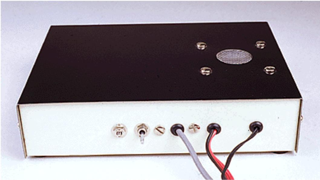
Figure 6—The rear panel of the DF unit supports the two DPDT **PHASE** toggle switches. Grommets in the panel holes allow abrasion-free passage of the antenna, dc-power and audio cables. The dc power cord is outfitted with an inline fuse holder and a male Jones plug. A six-pin female Molex connector (five pins are used) feeds the four antennas. The audio-input cable is terminated in a 1/8-inch diameter male plug.
