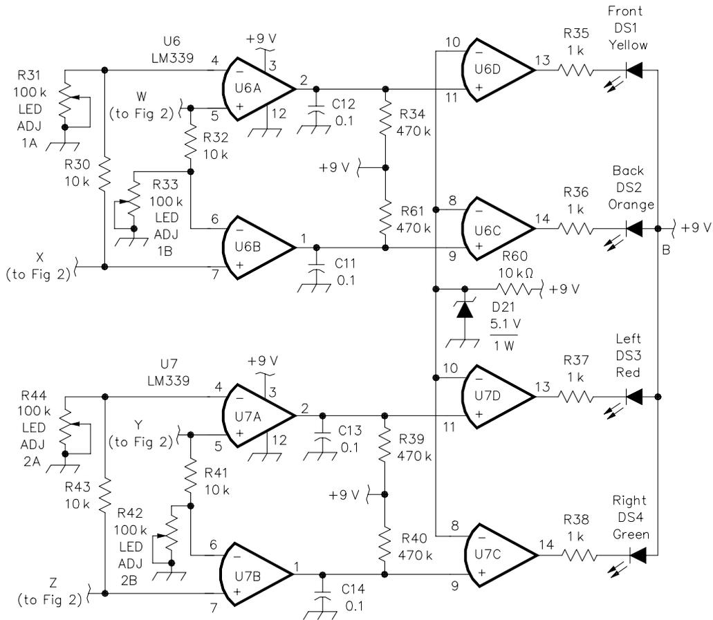
Figure 4—Schematic of the LED driver circuit. Part numbers in parentheses are Radio Shack. All fixed-value resistors are 1/4-W, 5%-tolerance units. Equivalent parts can be substituted.
