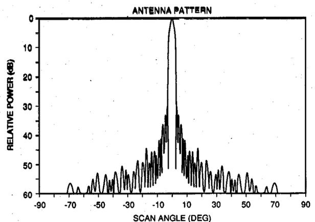
Figure 8a. Azimuth pattern in the shaped beam mode.
