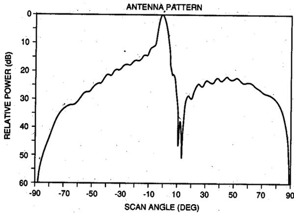
Figure 8b. Coscant-squared pattern in elevation plane.
