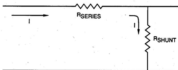
**Figure 4. Two-wire transmission line equivalent circuit of the waveguide slot radiator.**
