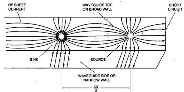
Figure 2. Sheet current flow pattern in a waveguide.
