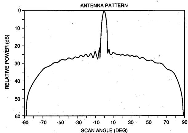
Figure 7b. Elevation pattern in the pencil beam mode.
