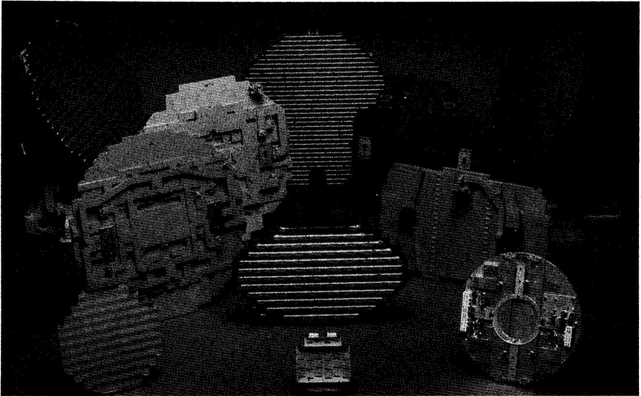
Figure 1. Flat-plate antennas for airborne applications (photo courtesy of Rantec Corp.)
