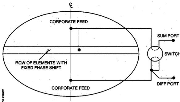
Figure 9. Simplified schematic of beam shape switching technique showing RF switch in the coscant-squared mode position.
