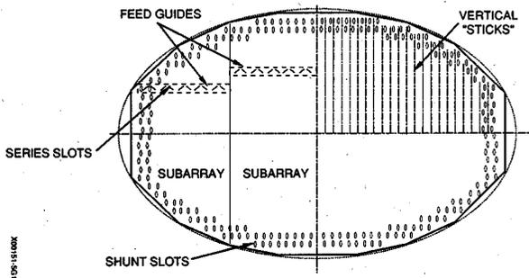
Figure 6. Typical flat-plate array showing shunt and series slots, as well as vertical stick radiating guide sections driven by a feed guide with series slots.
