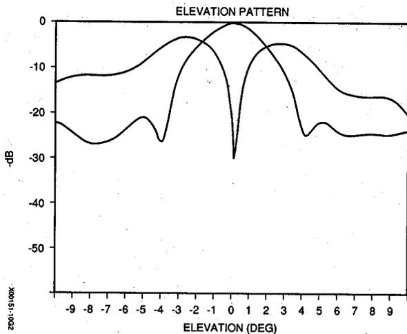
Figure 10. Superposition of the elevation sum and difference patterns.
