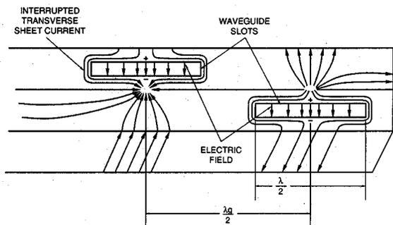
**Figure 3. Shunt radiating slots cut into the broad wall of waveguide.**
