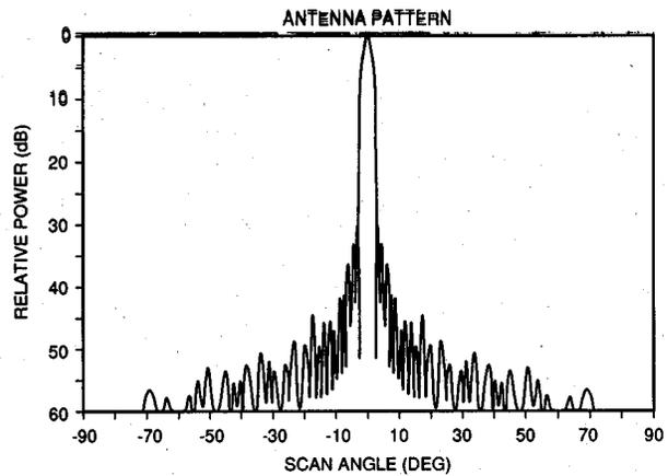
Figure 7a. Azimuth pattern in the pencil beam mode.
