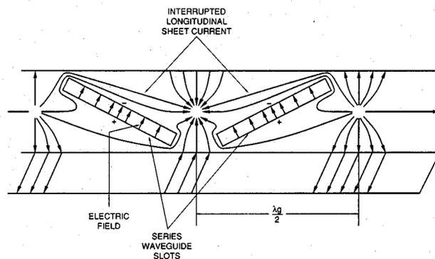
**Figure 5. Series slots cut into the broad wall of the waveguide.**
