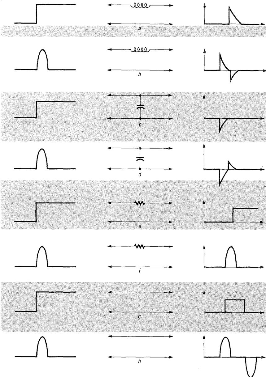
FIG. 4—SHARP PULSES are fed to inductive (a), capacitive (c), resistive (e), and straight-through (g), conductors. Half-sinewaves are fed to corresponding circuits in b, d, f and h.
