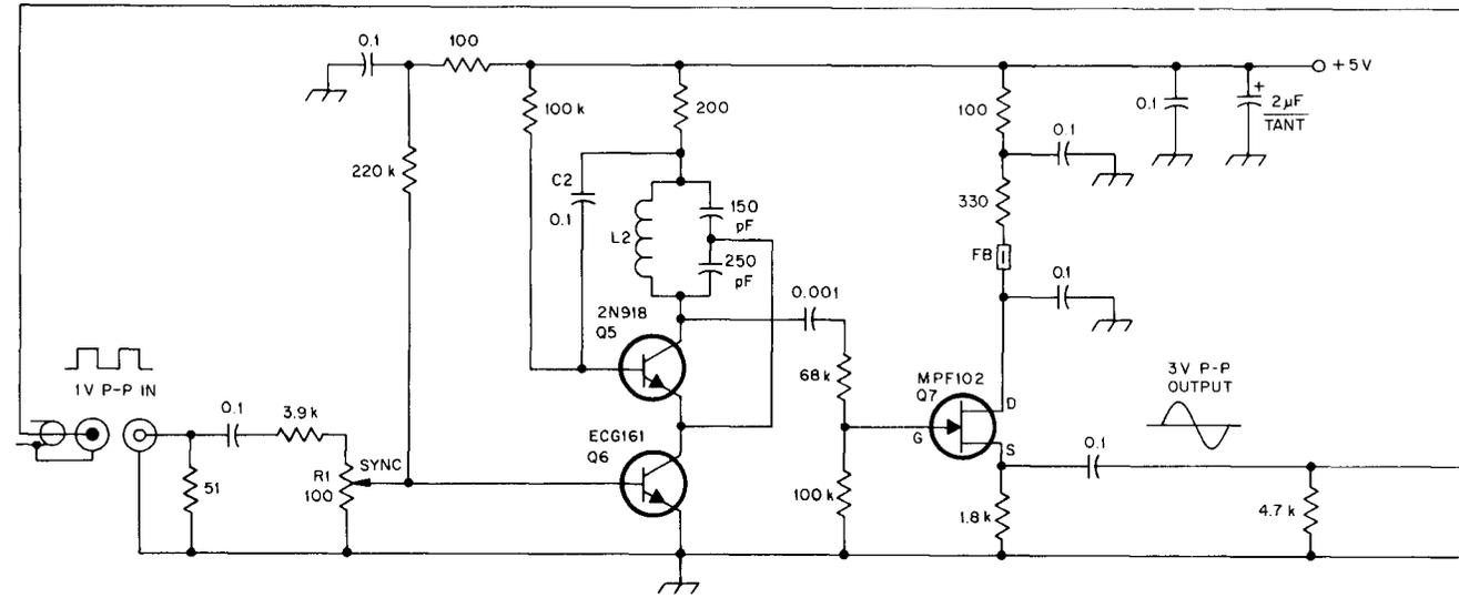
**Fig 3**—This circuit extracts stable clock signals from AM broadcast carriers for amateur spread-spectrum applications. All 0.1- $\mu$ F capacitors in coupling and decoupling circuits are miniature 50-V polyester types. All capacitors smaller than 0.1- $\mu$ F are silver mica.
