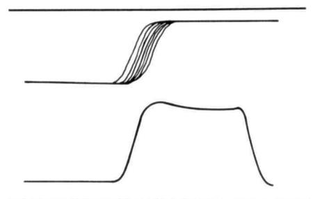
Fig 7—The upper trace shows the input signal going to the synchronized oscillator, and the lower trace is the signal at the emitter of Q8. The vertical scale is 1/div; the horizontal scale is 0.02  $\mu$ s/div.
