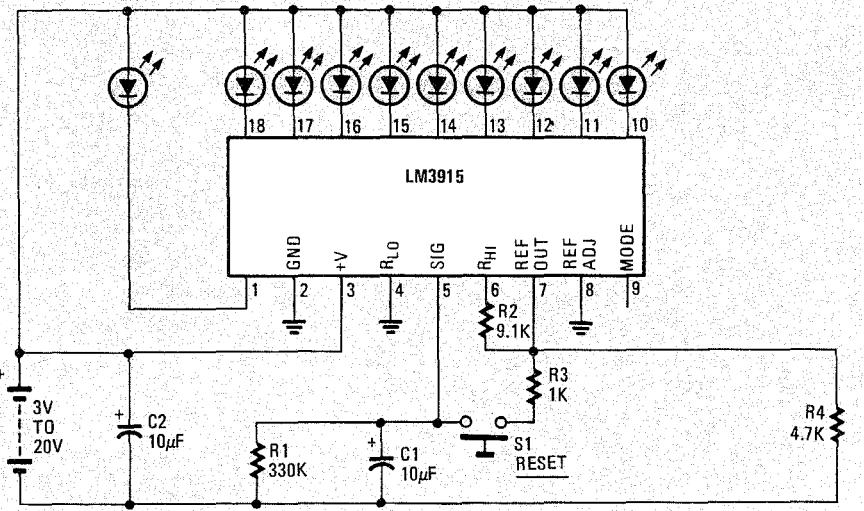
FIG. 8—TEN-STEP TIMER CIRCUIT. The LED's turn off sequentially, with each LED representing the time constant of  $R1-C1$ .
