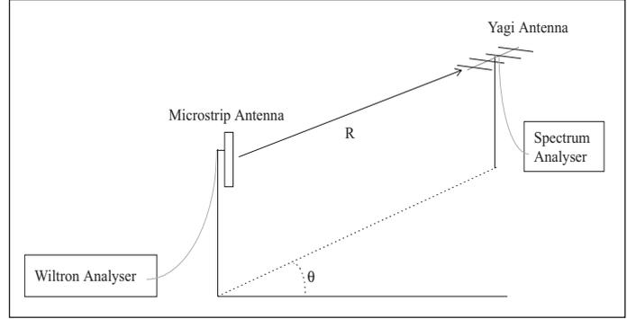
■ Figure 3. Antenna gain and polar pattern measurement setup.
