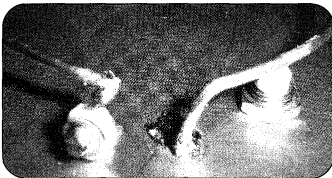
Photo I. Using a capacitor to lower the DDRR's frequency.
