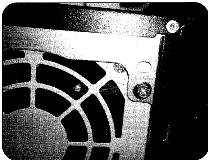
Photo F. An unintentional slot antenna—a computer case.
