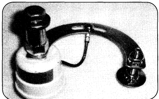
Photo C. A commercial 440-MHz vertically polarized DDRR antenna.
