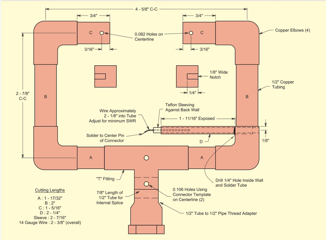
Figure 3—Constructional details for the 440 MHz antenna.
