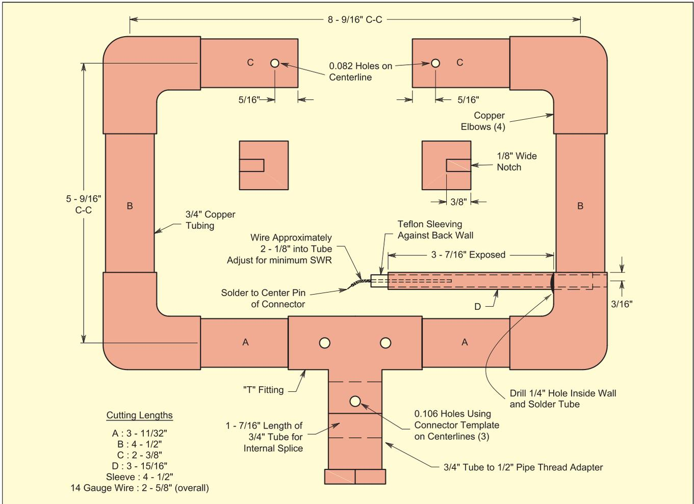
Figure 2—Assembly information for the 222 MHz loop antenna.
