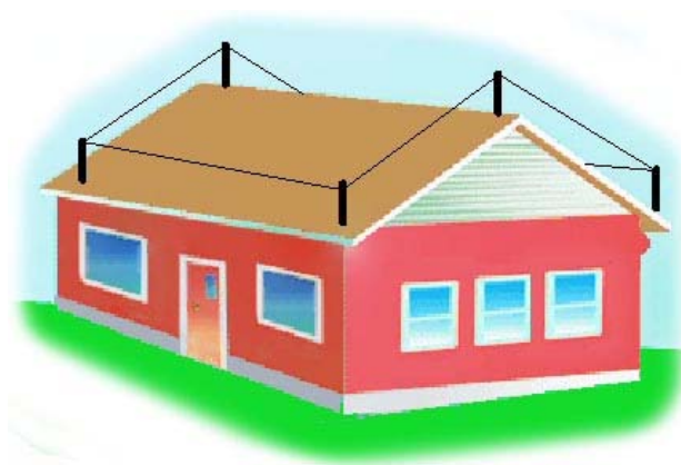
Figure 1: Classic rain-gutter-height loop, elevated on standoffs (stylized for emphasis)
