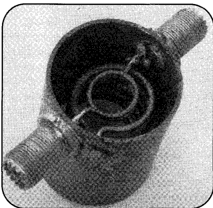
Bottom view of the filter. The author suggests attaching the coax connectors to the tube with brass screws and nuts, rather than trying to solder them on, as he did. Note the smaller coupling coil and capacitor connected between the coax connectors.
