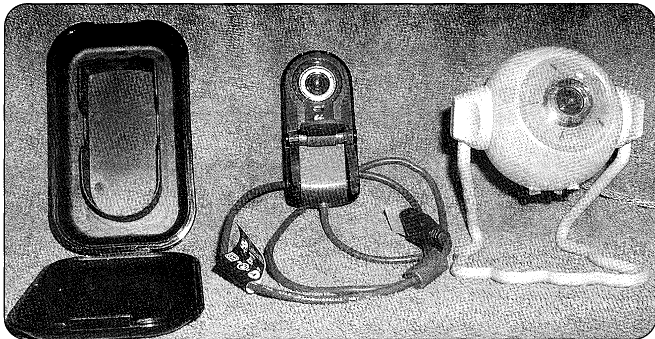
On the left is the Logitech USB 1.1 Notebook Pro camera and its carrying case (for information see < http://www.logitech.com >). The large golf-ball camera on the right is the Orange Micro iBOT2, a USB 2.0 version of Logitech's iBOT firewire camera (for details see < http://www.orangemicro.com >). (Photo courtesy AH7R)
