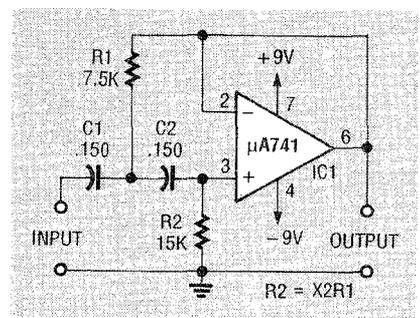
FIG. 6—A UNITY-GAIN, SECOND-order, 100-Hz high-pass filter.
