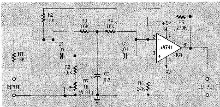
FIG. 15—A TWIN-T 1-KHz NOTCH FILTER with shunt feedback.
