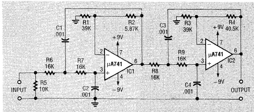
FIG. 5—A FOURTH-ORDER LOW-PASS FILTER for 10-kHz signals.
