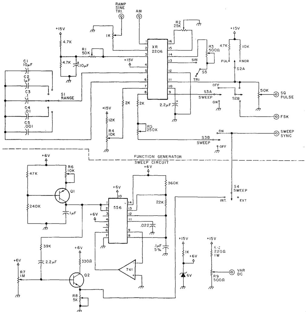
Fig. 1. Schematic of function generator and sweep generator.
